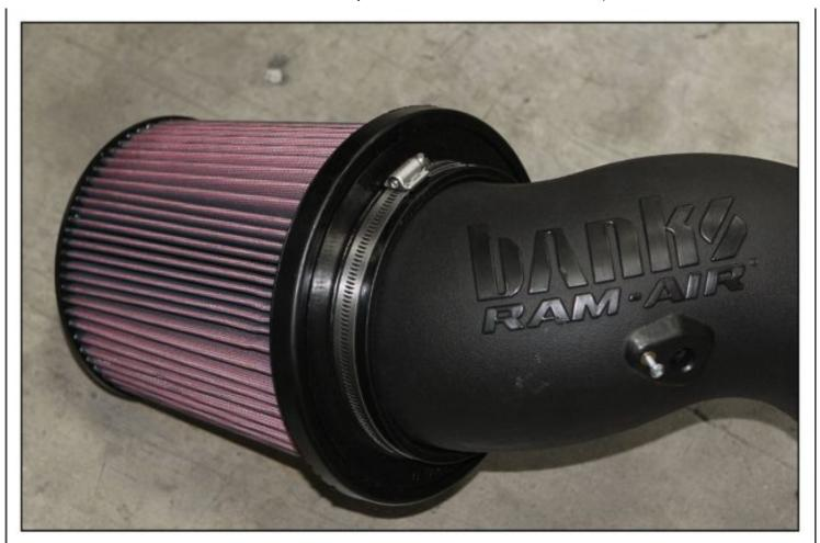
16. Install the Banks Ram-Air Filter onto the Intake Tube and secure it with the hose clamp. The hose clamp must be held up against the base of the filter while tightening the clamp.
