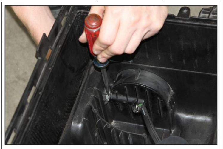
10. Using a flat blade screwdriver inserted between the Ram-Active Air® door and the side of the housing gently pry the door from the actuator motor shaft and pull the actuator motor from the housing.
