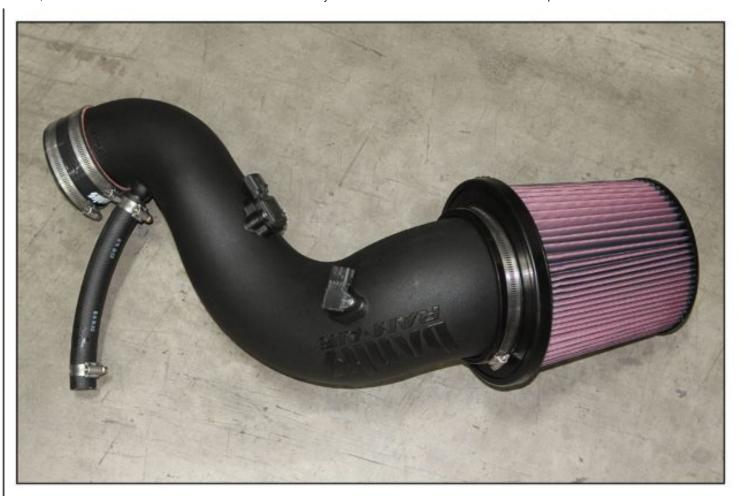
14. Remove the IAT and MAF sensors from the stock intake using a 7mm socket. Replace MAF sensor O-ring with supplied 3.5mm O-ring. Install these sensors in the Banks Intake Tube using the supplied screws and a Phillips screwdriver.
