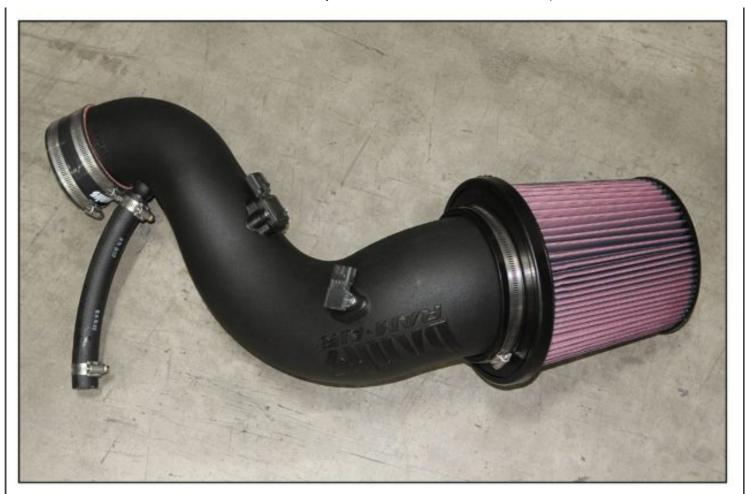
15. Install the PCV hose and two hose clamps along with the compressor inlet hose and its two hose clamps onto the Banks Intake Tube in the orientation shown in the picture. Tighten the clamps retaining the hoses to the tube and leave the other clamps loose.
