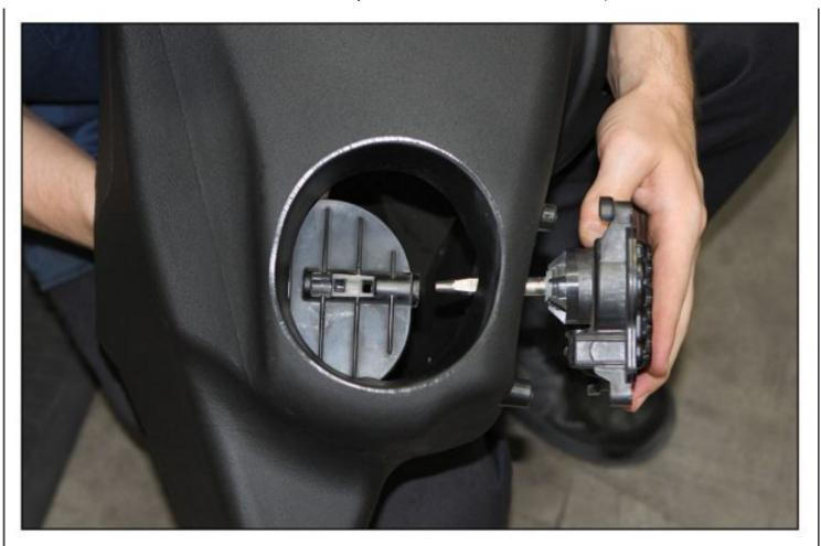
12. Install the Ram Active Air® and actuator motor into the Banks housing. Begin to insert the actuator motor from the side and hold the door over the actuator motor shaft.
