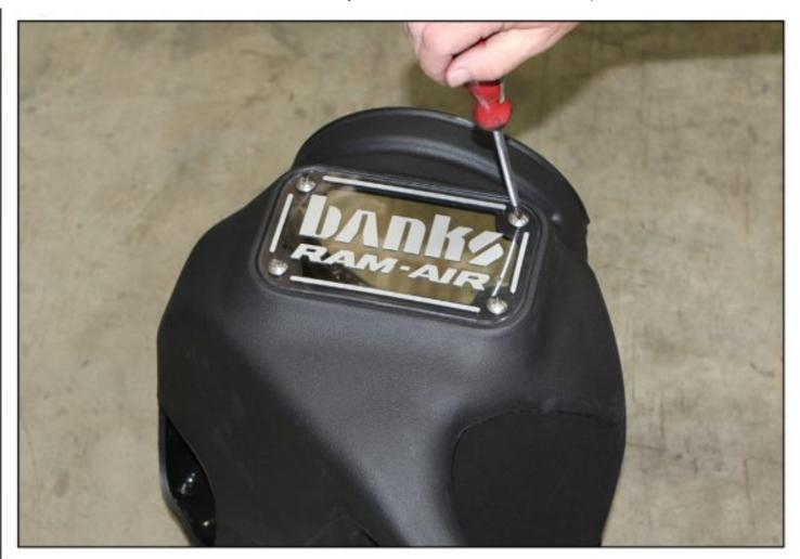
17. Apply blue thread locker to 4 supplied window screw and use to install clear window onto the housing. Do not overtighten the screw. They just need to be snug.
