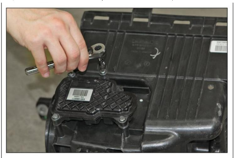
9. Remove the four screws retaining the actuator motor on the side of the housing using a T-30 Torx driver.
